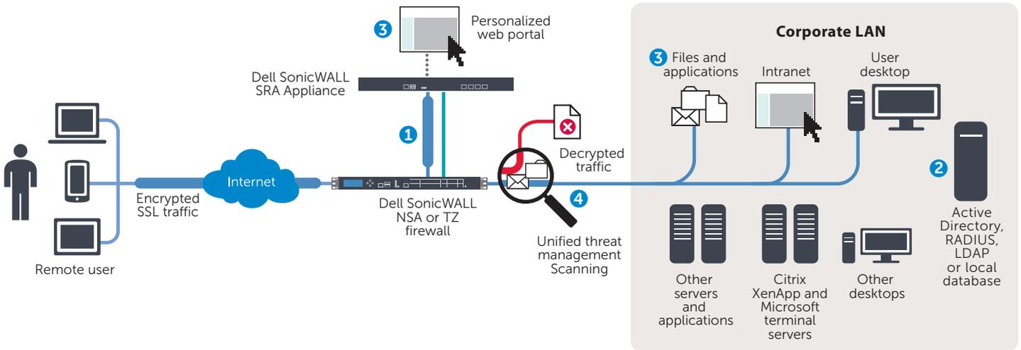
1 Incoming HTTPS traffic is seamlessly forwarded by the Dell SonicWALL NSA or TZ Series firewall to the Dell SonicWALL SRA appliance, which decrypts and authenticates network traffic.
